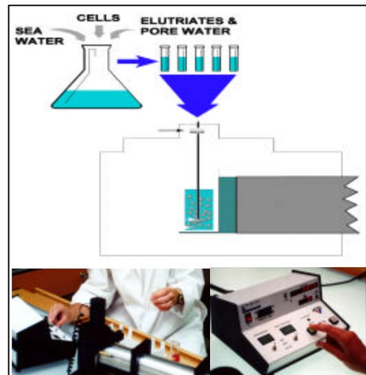
Figure 2. Schematic of toxicity test setup and the QwikSed toxicity unit.
