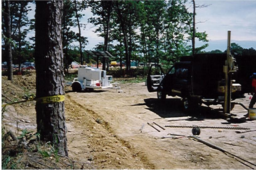
Figure 11. SEAttrace™ System remotely operated on site at the Viscous Liquid Barrier (VLB) test site in Brookhaven, NY (background). In the foreground, completion of the vapor sampling point installation can be seen.
