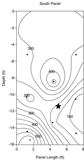
**Figure 9. Tracer concentration profiles and inferred leak location (star) created by the 12-inch hole that was drilled horizontally through the south panel of the Deep Active Box. Vapor monitoring ports are indicated by solid black circles.**
