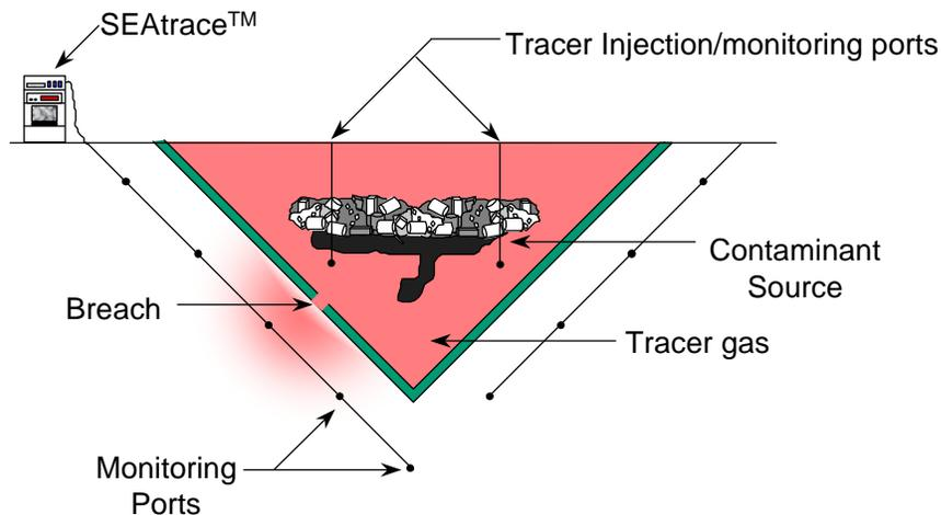
Figure 1. Schematic of the SEAttrace™ System
