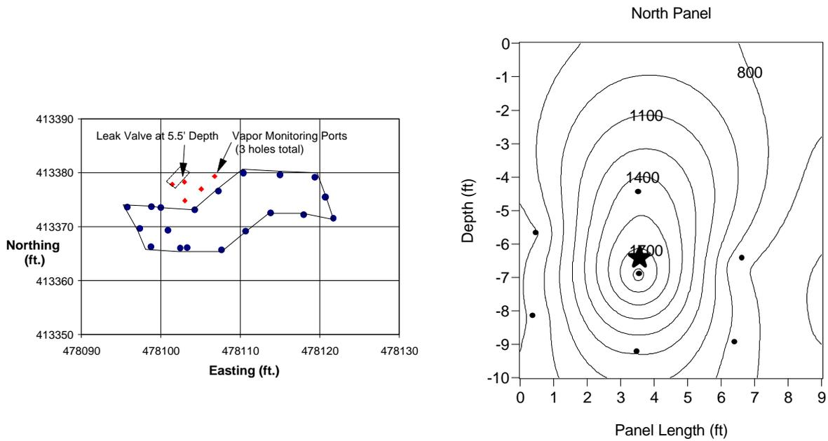
**Figure 8. Leak anomaly configuration (adjacent to shallow passive test box) and concentration data showing inferred leak location (star) adjacent to vertical panel section. Black circles on schematic to right denote vapor sampling port locations.**
