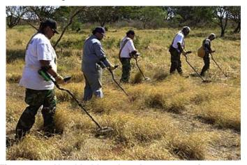
Figure 3-18. Hand-held analog electromagnetic systems.
