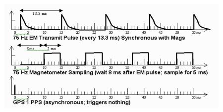
Figure 3-16. Interleaving of magnetometer and EMI measurements in dual-mode timedomain system. The top trace shows EMI pulse, center trace shows magnetometer detection window, bottom trace shows operations clock that governs overall system timing.
