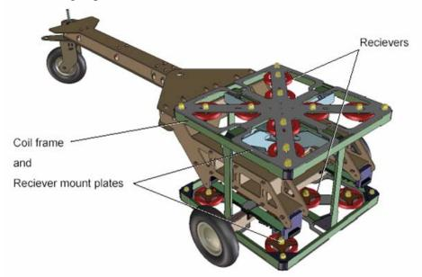
Figure 7-5. Field prototype of multisensor active electromagnetic system.
