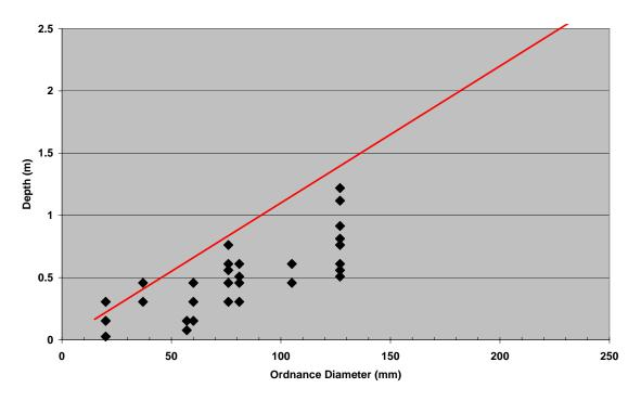
Figure 4-9. ADAK GPO seed items depth versus munitions size. (Depth distributions that include few or no items below the  $11\times$  line are typical.)
