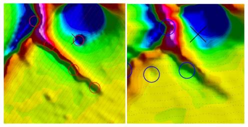
Figure 6-1. The target marked by the X is a mortar. The demonstrator on the left, with closer track spacing, is able to resolve the target of interest from the nearby large clutter object and marks it with a circle. The demonstrator on the right, with larger line spacing, is not.
