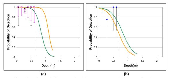
Figure 5-24. Detectability versus depth for 60 mm mortar for better performing magnetometer and EM sensors at selected GPOs. The lines are fits to the Pd-by-depth data from the Standardized Test Sites: green = APG, orange =YPG. (a) shows the EM61Mk1 (black) and EM61 Mk2 (pink); (b) shows the magnetometers. The dashed vertical line indicates the 11× depth.
