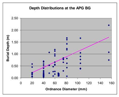
Figure 4-4. Depth distributions in the APG Blind Grid. The solid line shows depth =  $11 \times$  diameter. Note the large number of targets of all types buried at greater depths.
