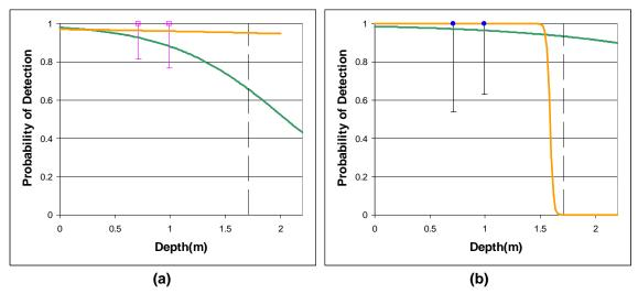
Figure 5-27. Detectability versus depth for 155 mm projectile for better performing magnetometer and EM sensors at selected GPOs. The lines are fits to the Pd-by-depth data from the Standardized Test Sites: green = APG, orange =YPG. (a) shows the EM61Mk1 (black) and EM61 Mk2 (pink); (b) shows the magnetometers.
