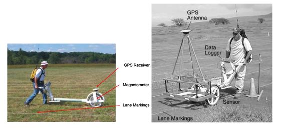
Figure 3-20. Examples of cart-mounted systems with cesium-vapor magnetometer sensors (left) and EM61 EMI sensors (right).
