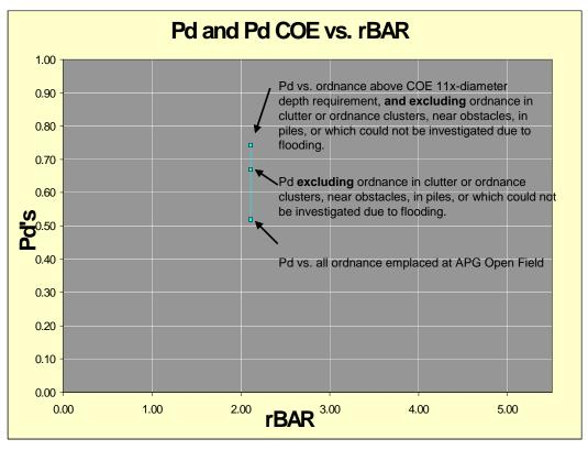
Figure 4-6. Example of standardized test site performance presentation. Pd is plotted against BAR. Good performers have high Pd and low BAR.
