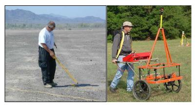
Figure 3-1. Schonstedt magnetometer (left) and Geonics EM61-MK2 EMI (right).
