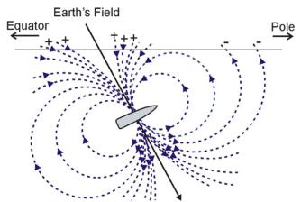
Figure 3-10. Perturbation of Earth's field by ferrous ordnance.
