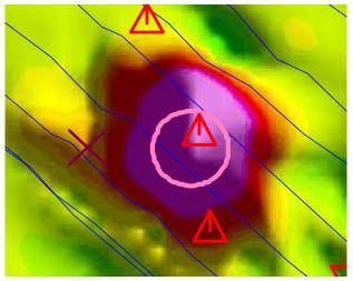
Figure 5-14. Example of overlapping signatures. A 40 mm projectile at 0.4 m (marked with the X) is 1.5 m distant from an approximately 1 kg clutter item at 0.05 m depth marked with the red triangle).
