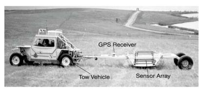
Figure 3-21. Towed sensor array platform.
