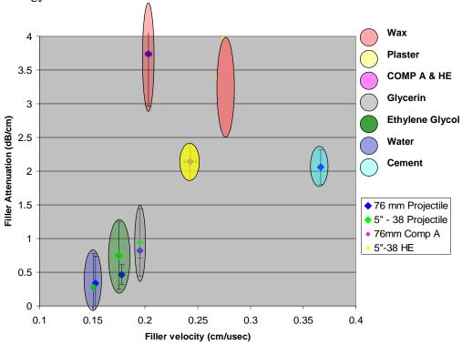
Figure 8-2. Attenuation versus acoustic velocity cluster plot.
