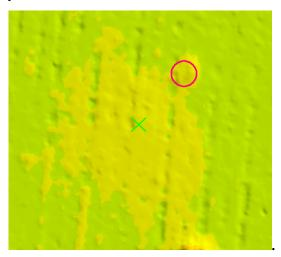
Figure 5-16. Better demonstrator miss of a 155 mm projectile at depth 1.6 m (marked with X). The item is just less that 11× its diameter in depth, and the nearest alarm (circle) is several meters away.
