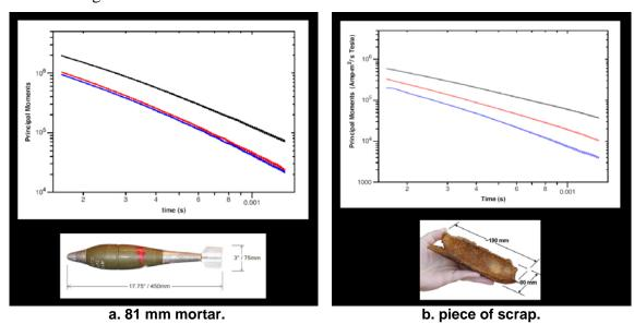
Figure 7-3. Lawrence Berkley National Lab model results for the principal polarizability moments as a function of decay time calculated for a munitions item and a piece of scrap.
