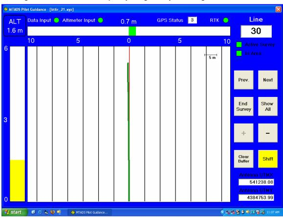
Figure 3-25. Screen shot of a towed-array navigation system based on DGPS.
