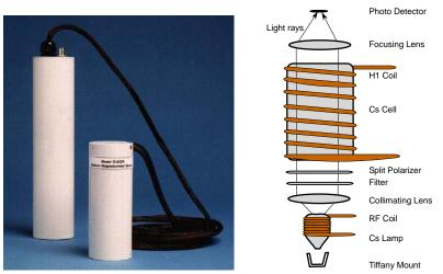
Figure 3-13. Photo and diagram of G-858 cesium-vapor magnetometers.
