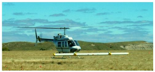
Figure 7-8. NRL Airborne MTADS magnetometer system.
