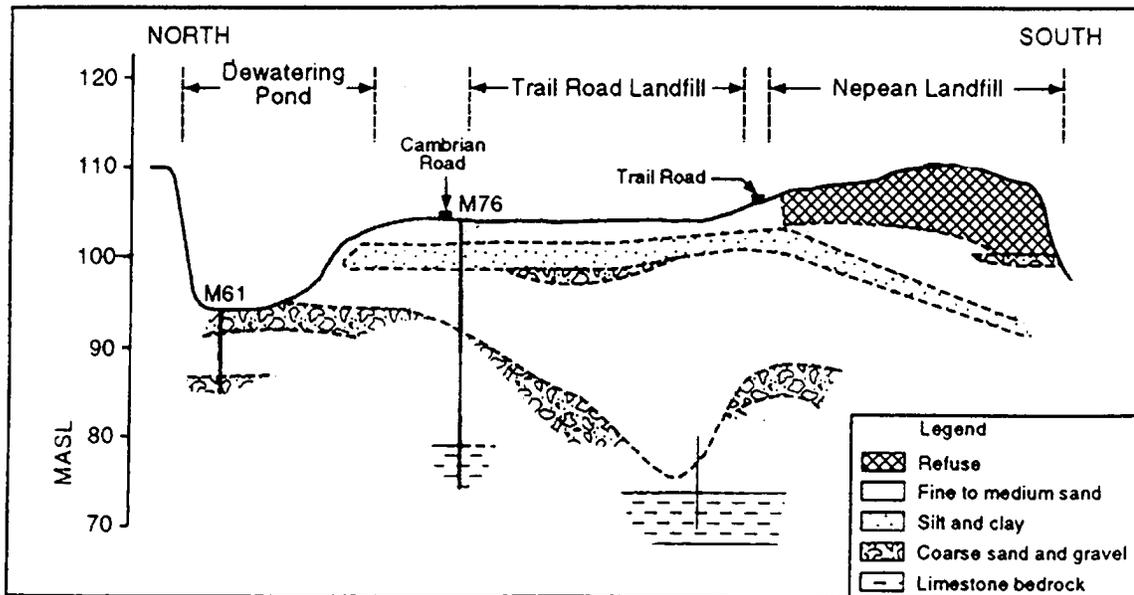
**Figure 2: North to South Cross Section of Site [3]**
