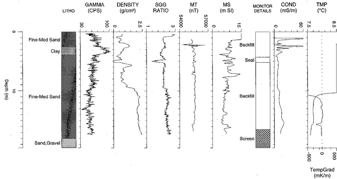
Figure 4: Geophysical Log for Well M83 [5]
