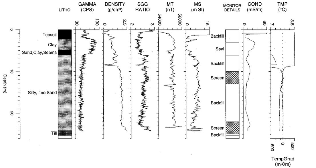
Figure 5: Geophysical Log for Well M76 [5]
