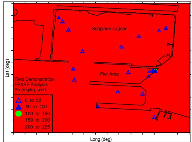
Figure 3. Contaminant distribution model based on XRF data shows good correlation with data in Figure 4.
