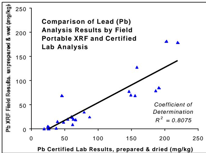
Figure 2. Close correlation in the comparison of XRF and lab results on split samples.
