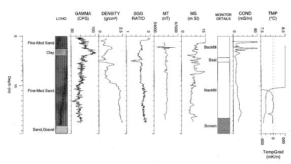
Figure 4: Geophysical Log for Well M83 [5]
