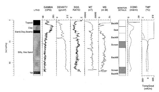
Figure 5: Geophysical Log for Well M76 [5]
