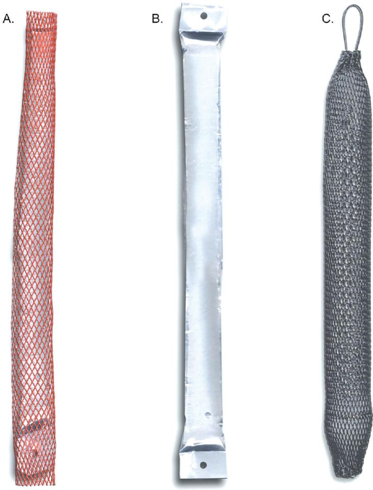
**Figure 1.** Typical water-filled passive diffusion bag samplers used in wells, including (A) diffusion bag with polyethylene mesh, (B) diffusion bag without mesh, and (C) bag and mesh attached to bailer bottom.
