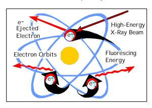
*Figure 1. Physics of x-ray fluorescence technology.*
