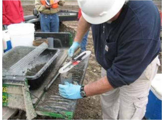
Figure 6-2. Field preparation of cylinder molds of freshly treated material. Source: Ed Bates.
