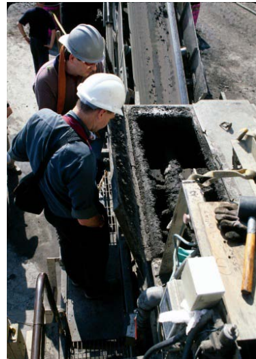
Figure A-4. Pugmill mixer trough opened showing mixing paddles at Peak Oil Co./ Bay Drum Co. Superfund Site, Tampa, Florida. Source: Portland Cement Association.
