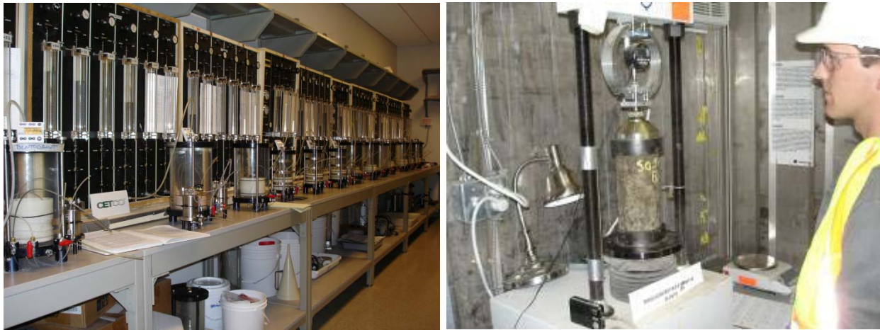
Figure 5-1. Hydraulic conductivity measurement (left) and UCS measurement (right) tests conducted in the laboratory on treatability test samples. Source: CETCO Contracting Services Co.
