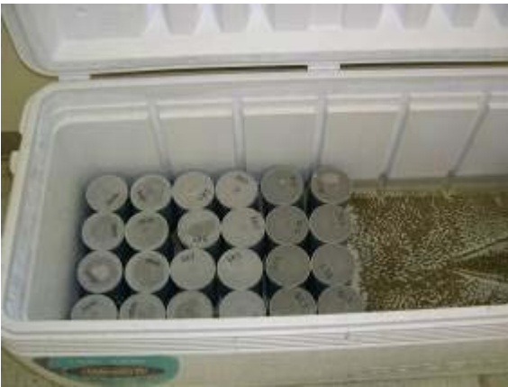
Figure 6-6. Field curing of S/S material specimens in a humid atmosphere (water bath). Source: Ed Bates.
