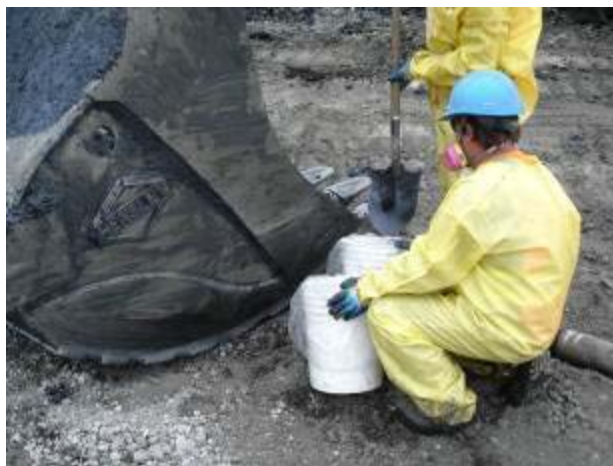
Figure 6-4. Sample collection of freshly mixed material from an excavator bucket. Source: CETCO Contracting Services Co.
