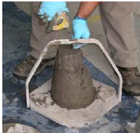
Figure 6-7. Slump test on freshly treated material. Source: Ed Bates.
