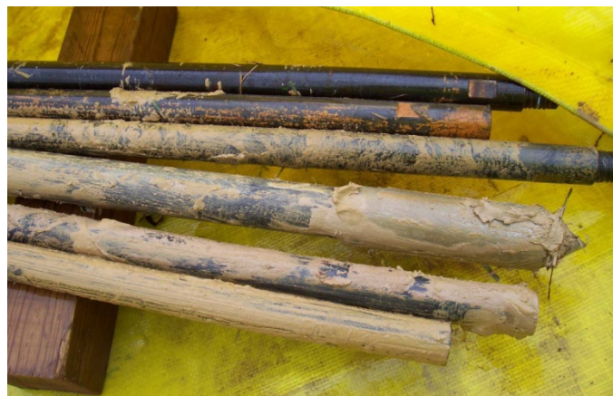
Figure 4-3. Clogged Injection Tooling
