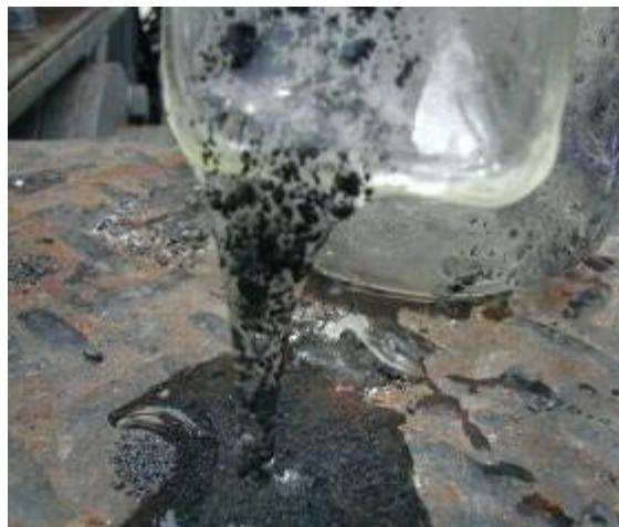
Figure 6-9. Fine-grained iron injected in a guar suspension.
