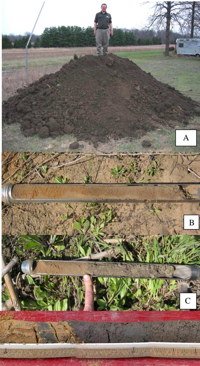
Photo 1. Soil materials used at the Sand Farm research site; A, sediment as delivered to site; B, Bloomfield Sand core showing thin, weak A horizon on right; C, Bloomfield sand core with 30 cm applied sediment; D, 30 cm sediment core showing some mixing at the interface.
