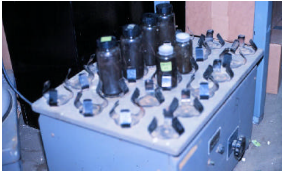
Figure 6-4. Photo of Sequential Batch Leachate Test setup
