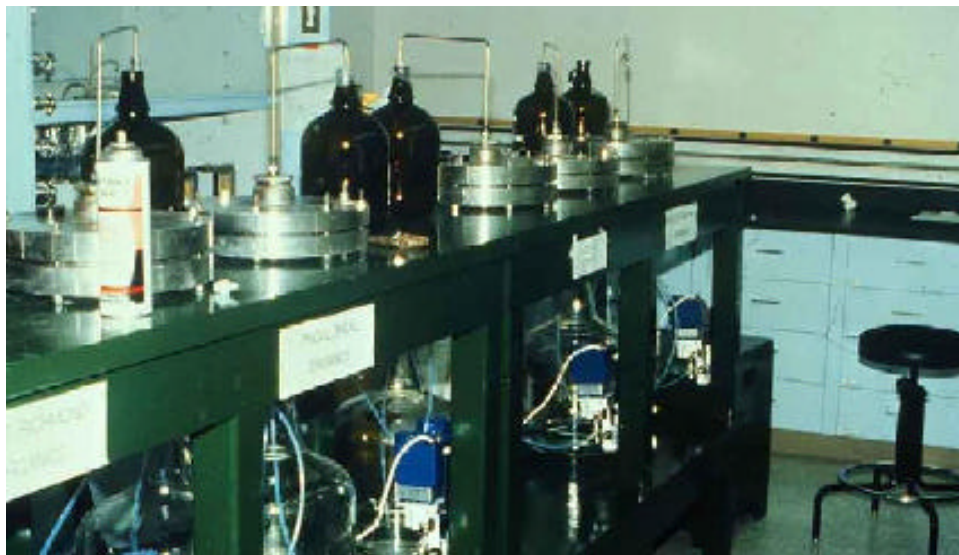
Figure 6-5. Photo of Pancake Column Leach Test setup
