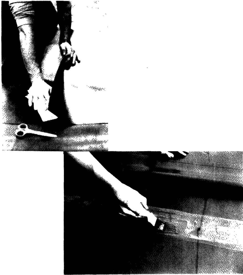
Figure 10.5(a). (Upper Left) Alignment of test strip and cleaning of area to be bonded.
