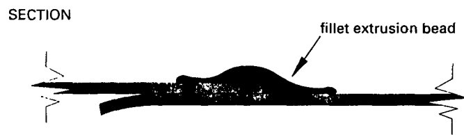
Figure 7.7. Hot wedge T-seam detail.
