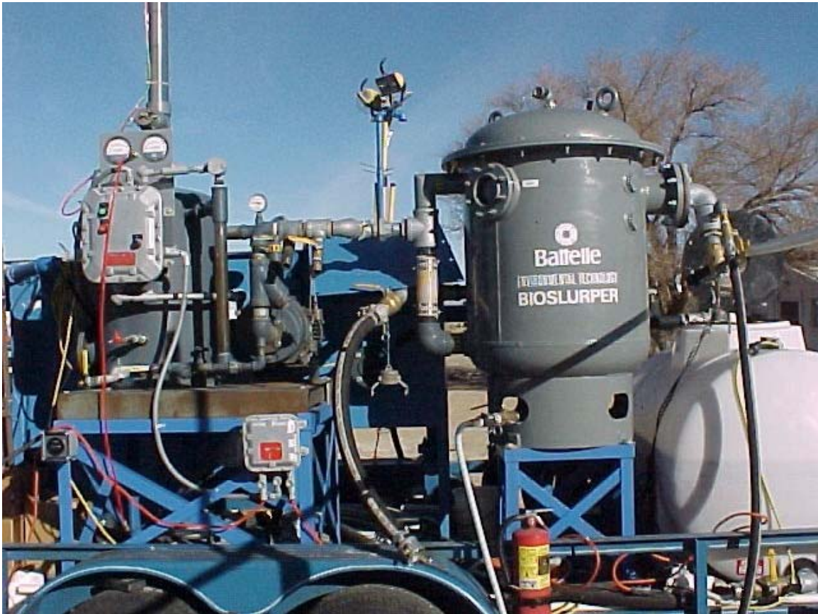
Figure 2-2. Vacuum-Resistant Separator on Mobile Bioslurper System
