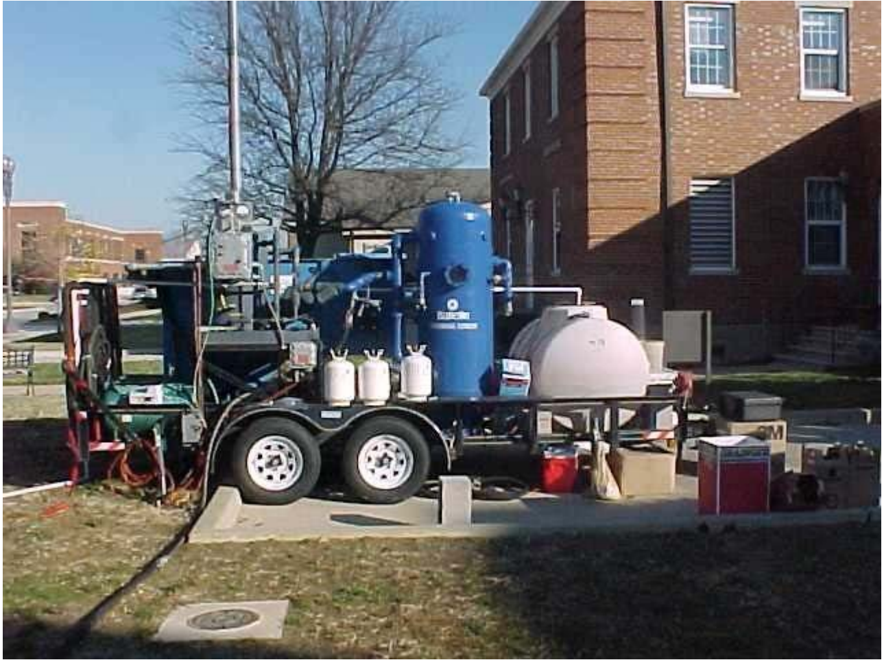
Figure 4-2. Photograph of Mobile Bioslurper System at Bolling AFB
