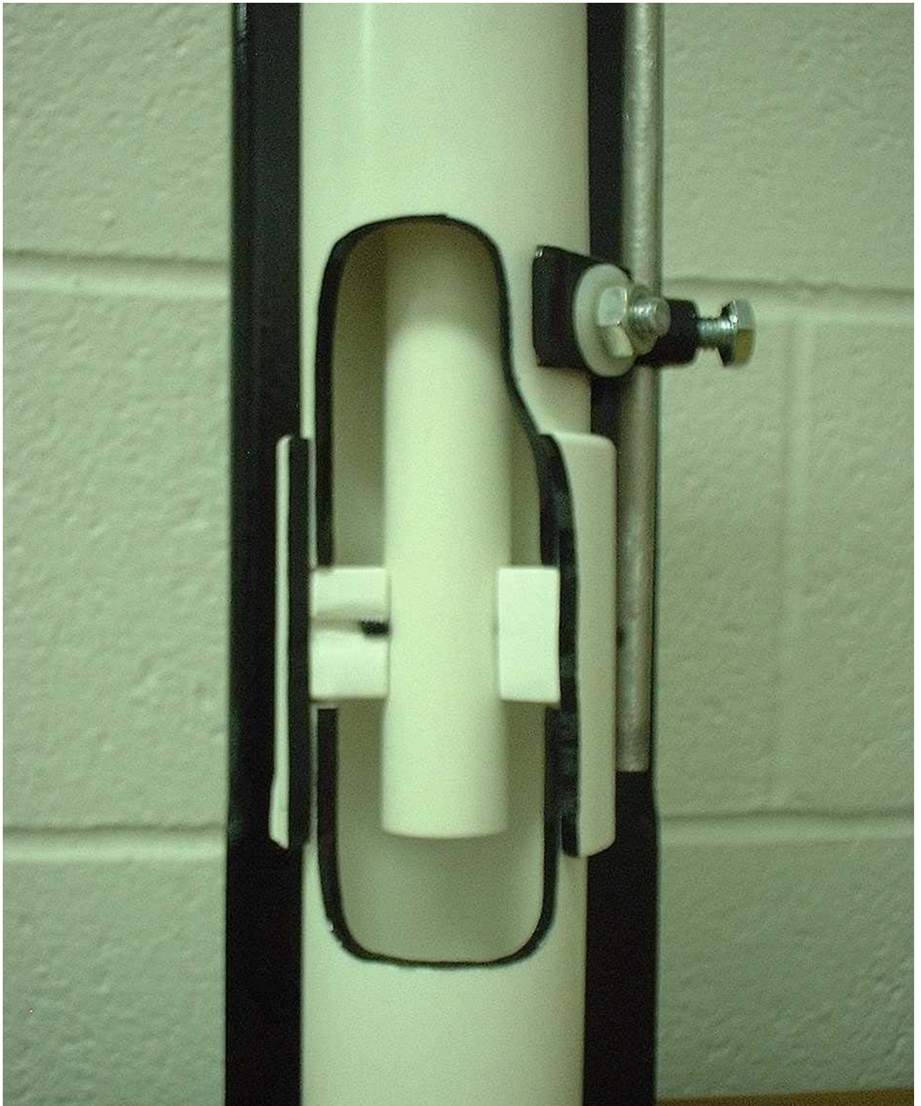
Figure 2-4. Photograph of the In-Well Pieces Dual Drop tube System Displaying the Soil Gas/Groundwater Drop tube, the Field Shield and The Fuel Extraction Drop Tube
