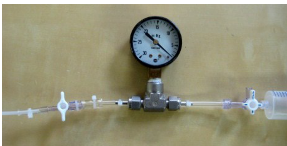
Figure G-11. Simple sampling train arrangement for a shut-in test using a syringe as the vacuum source.
