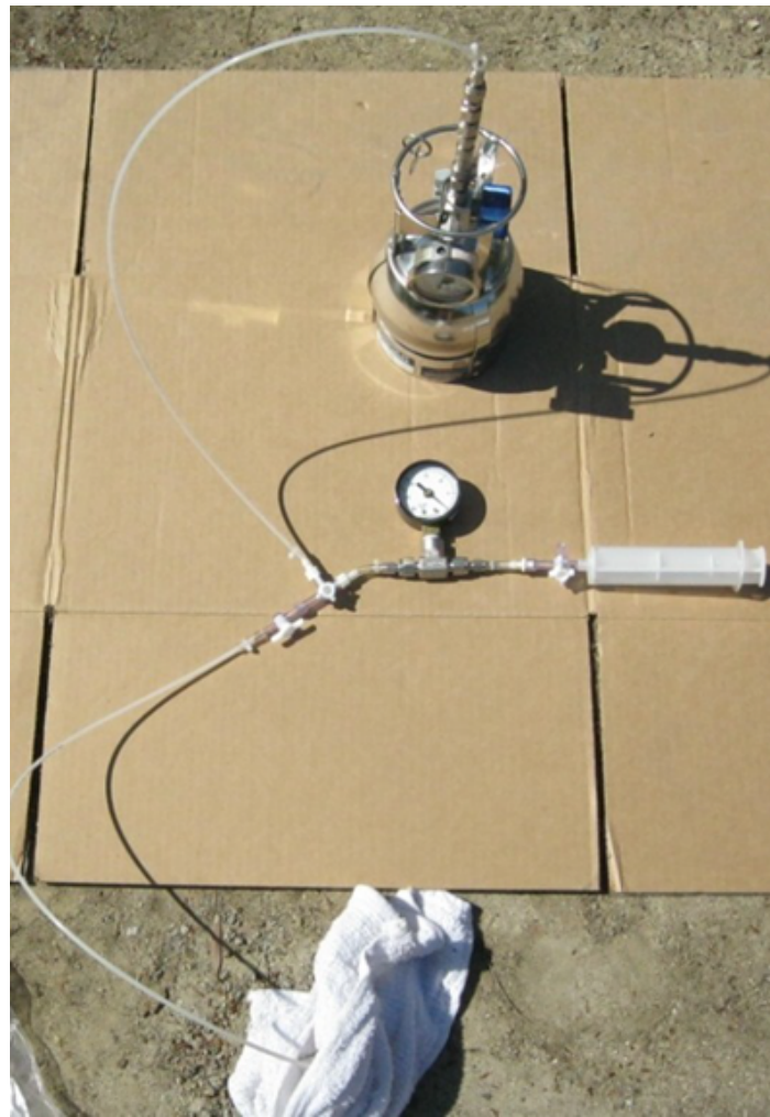
Figure G-12. Sampling arrangement showing probe tubing, leak check compound soaked into towel covering the probe at the ground surface.
