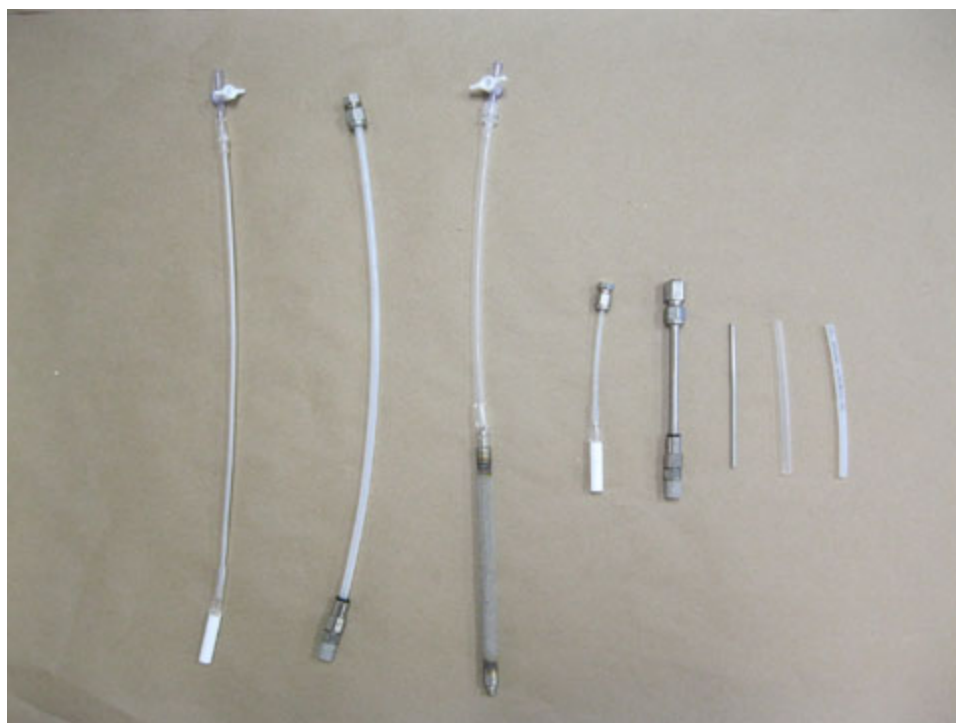
Figure G-9. Vapor sample materials, including 1/8-inch outer diameter tubing, three types of tips (ceramic, aluminum, and braided steel) and two types of surface terminations (stopcock and Swagelok fitting).
