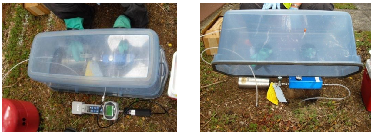
Figure G-14. Covering the entire sampling system and probe with a shroud.
