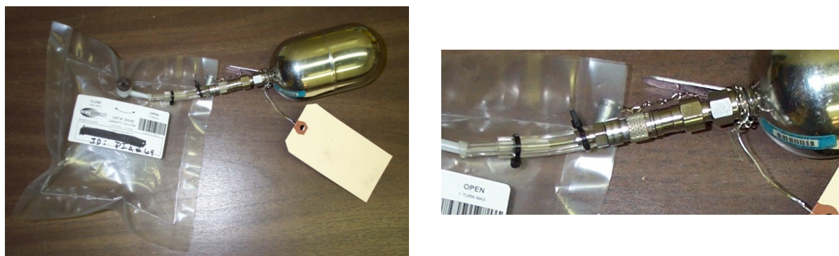
Figure G-16. Transferring soil vapor sample from a gastight bag into a 400 cc canister.
