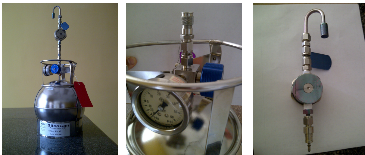
Figure G-1b. Sampling canister sampling assembly.
