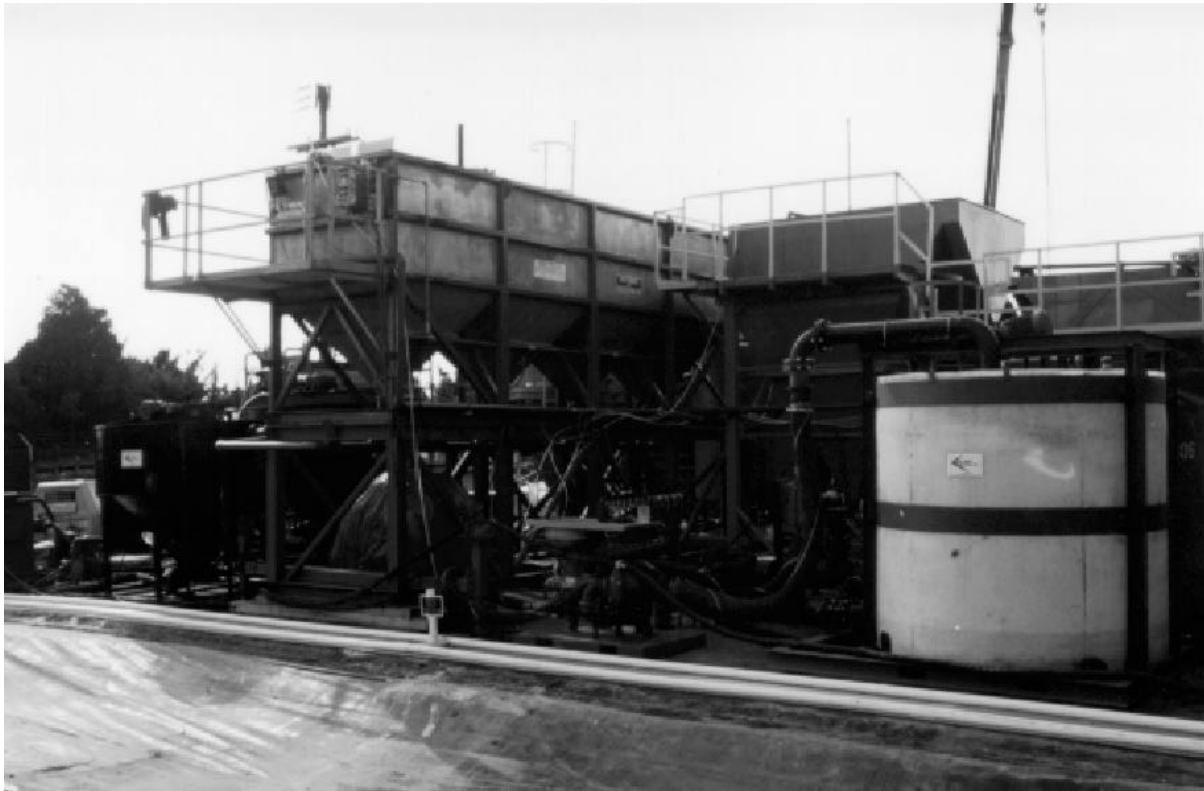
Figure 14. Baffled precipitation and settling tank on left forms part of Vendor 2's plant.
