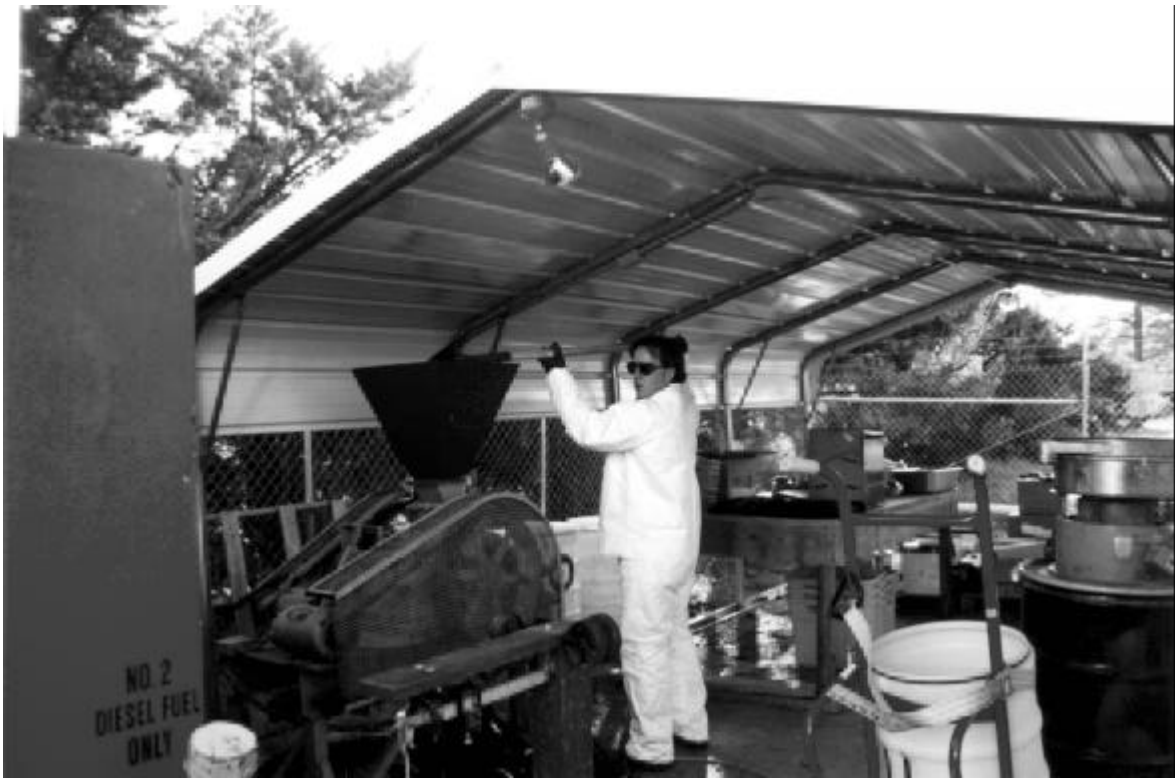
Figure 18. Covered sample preparation area with ovens, crusher, vibrating screen, and sample splitter.
