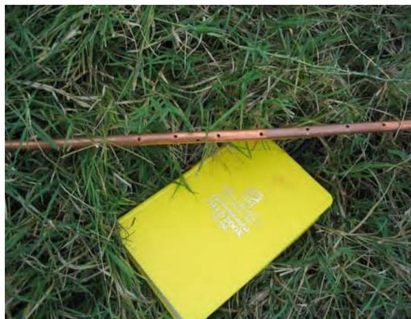
**Figure 6.1 Nitrogen Sprayer from Copper Tubing to Inject Liquid Nitrogen**
