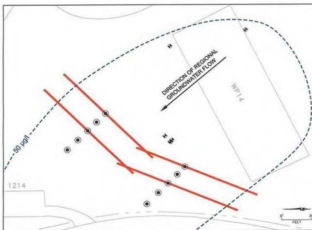
**Figure 3.1 Dual Biowall Configuration at Dover AFB, Delaware**
