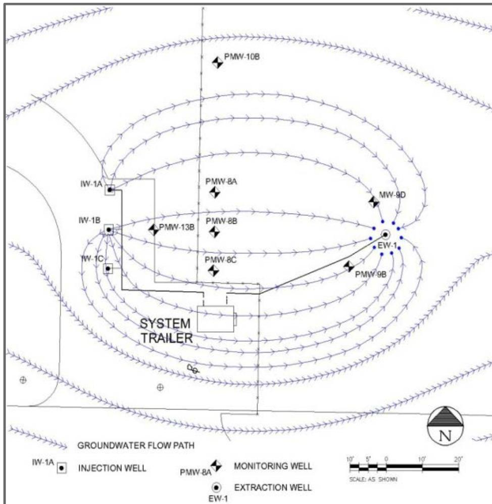
Figure 13. Typical Circulation System Layout (Kovacich and others 2006)
