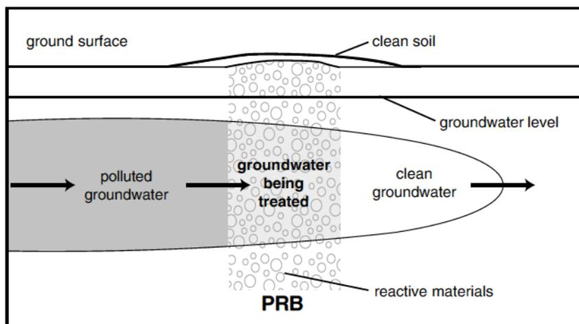
Figure 10. Permeable Reactive Barrier Example (EPA 2001b)
