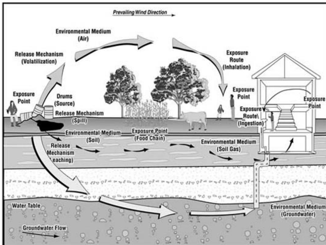
Figure 6. Conceptual Site Model - Exposure Pathway Schematic (ATSDR 2005)
