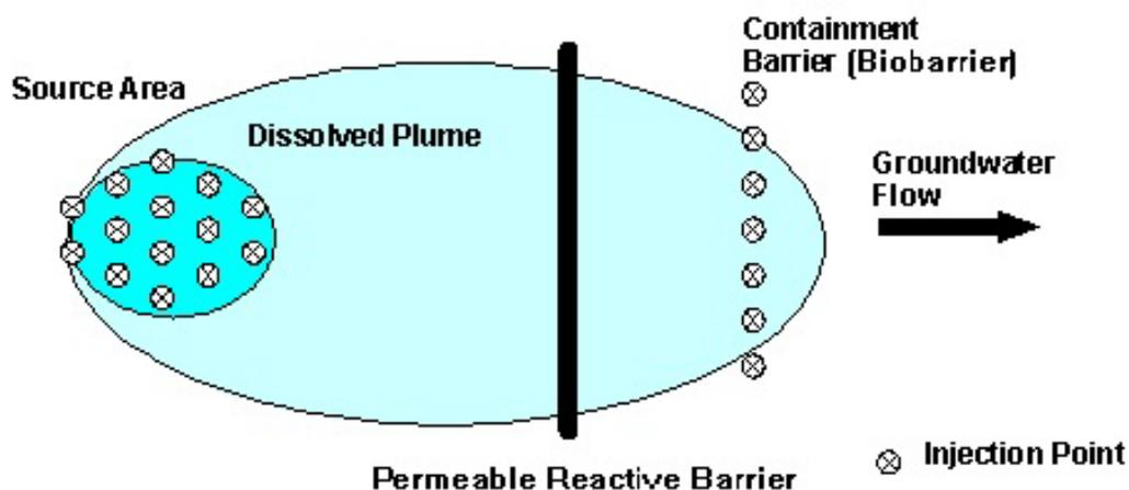
Figure 14. Schematic of Source Area and Barrier Injection Configurations.
