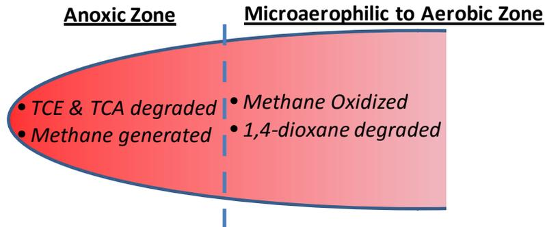
**Figure 3-1.** Schematic of two-phase treatment approach for 1,4-dioxane.
