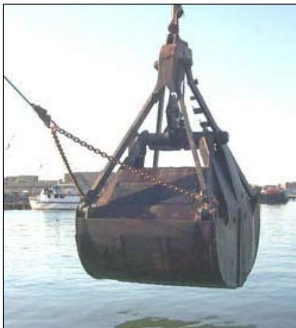
Figure 4-3. Enclosed Clamshell Bucket Prevents Escape of Sediment During Environmental Dredging
