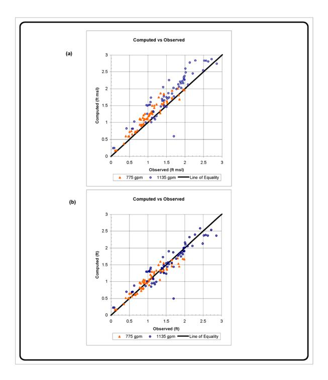
Figure B2-13. Summary of Drawdown Response to Pumping: Original Model (a) and Re-Calibrated Model (b)
