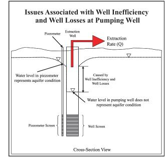
Figure 8. Issues associated with well inefficiency and well losses at pumping well.
