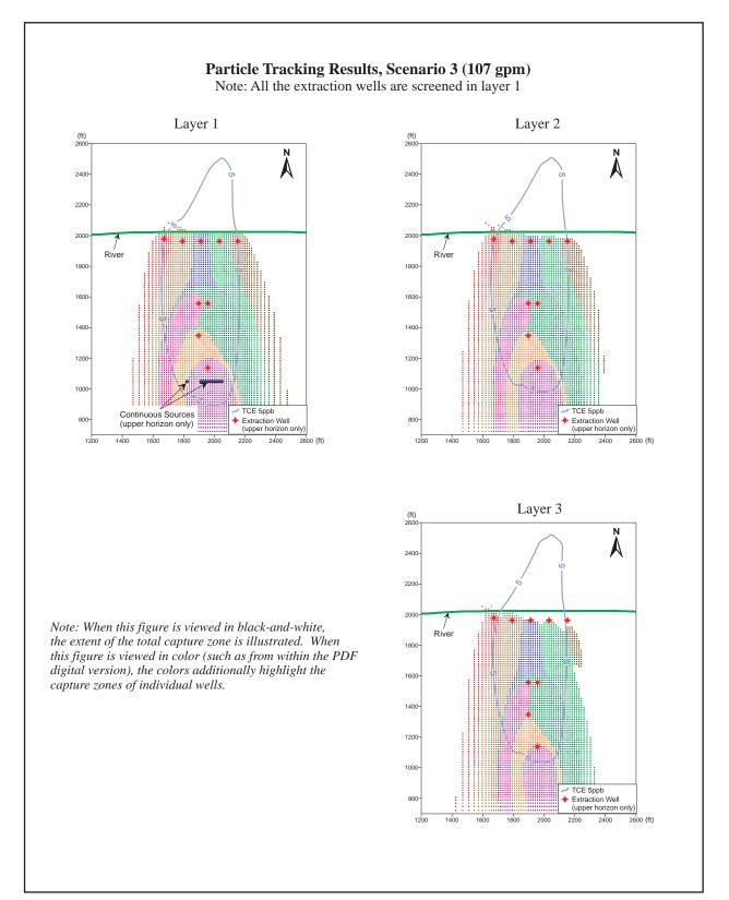
midpoint of Layer 1, Layer 2, and Layer 3 (i.e., each horizon of the shallow aquifer). No particles starting at the vertical midpoint of Layer 4 (the deep aquifer) are removed by any of the remedy extraction wells. Although these shallow extraction wells may help prevent contaminants from migrating down to the deep aquifer in the future, the particle tracking results indicate that they will not remove contamination that has already migrated down to the deep aquifer.
