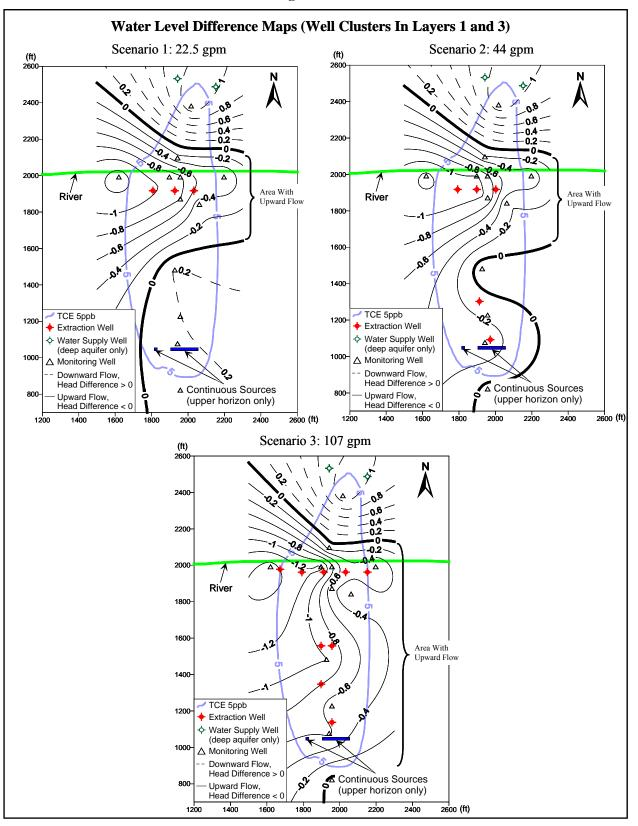
These vertical head difference figures were created by contouring the measured head differences from locations where water level data were available at multiple depths (i.e., clustered monitoring wells).
