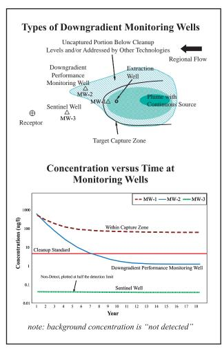
Figure 15. Types of downgradient monitoring wells.
