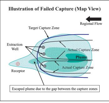
Figure 2. Illustration of failed capture.
