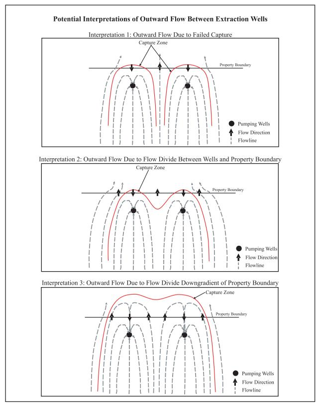
The capture zone width calculation and the particle tracking results for this example site (Figure A3-4) suggest that hydraulic containment is in fact achieved for Scenario 1, despite the outward hydraulic gradients observed between some water level pairs at the northern property boundary (Figure A3-5). To add conservatism, pumping rates could be increased to provide inward gradients at all water level pairs.
