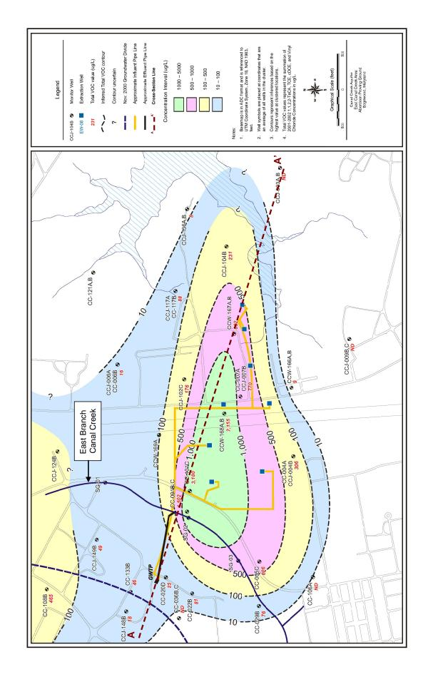
Figure B1-2. ECCA Study Area with VOC Plume and Extraction System
