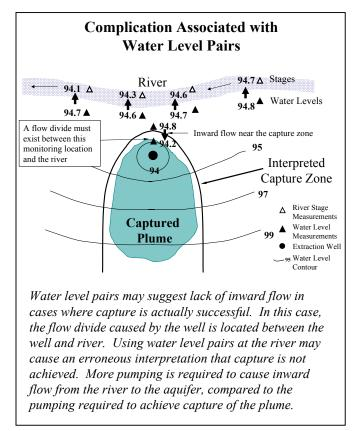
Figure 11. Complication associated with water level pairs.
