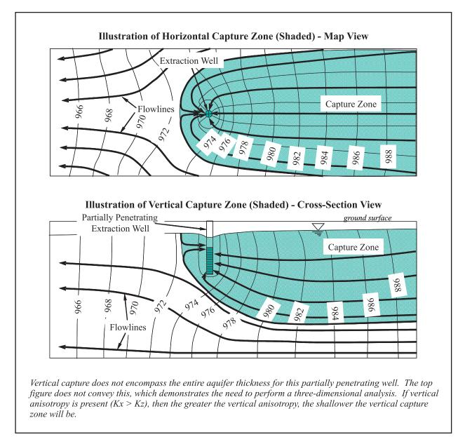
Figure 1. Illustration of horizontal and vertical capture zones.
