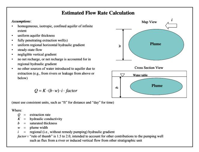
Figure 13. Estimated flow rate calculation.
