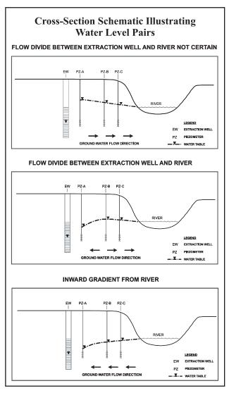
Figure 12. Cross-section schematic illustrating water level pairs.
