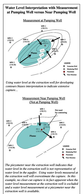
Figure 9. Water level interpretation with measurement at pumping well versus near pumping well.
