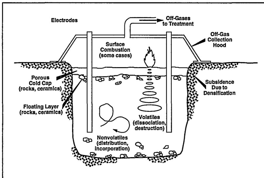
Disposition of Materials During ISV Processing
