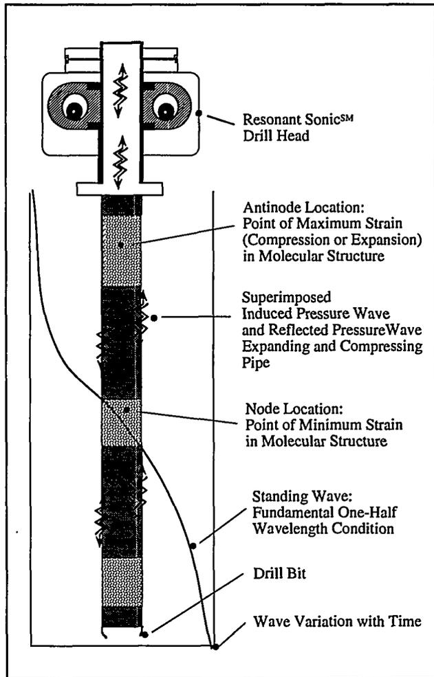
Figure 1. ResonantSonic<sup>SM</sup> Energy
