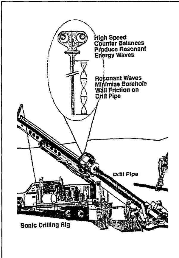
Figure 2. Schematic of ResonantSonic<sup>SM</sup> Drilling
