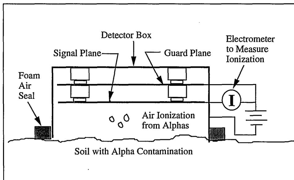
Figure 1. Schematic of the LRAD Soil-Surface Monitor
