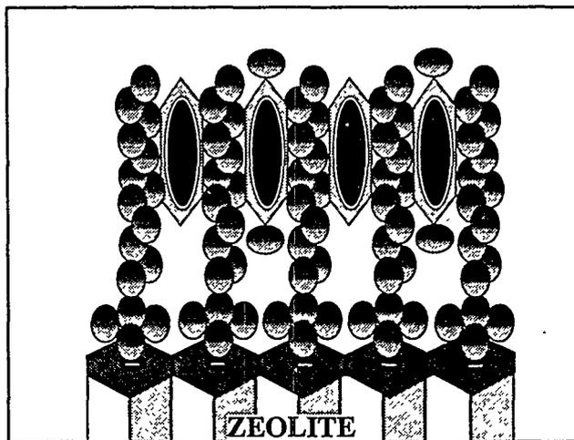
Figure 3. HDTMA-Zeolite Non-Selective BTEX Removal
