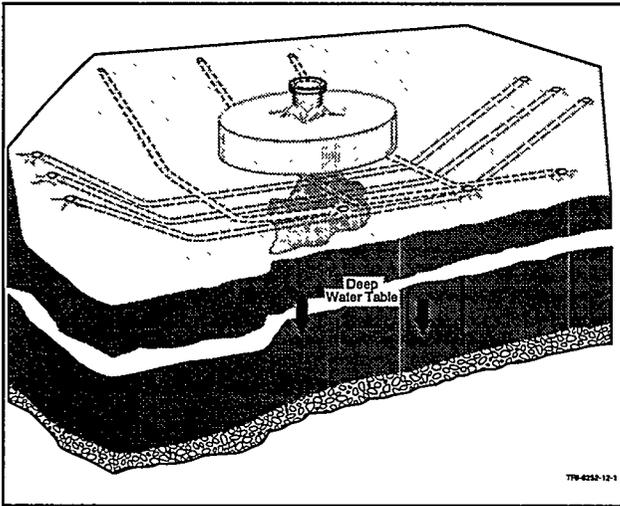
**Horizontal Wells Beneath A Buried Tank**
