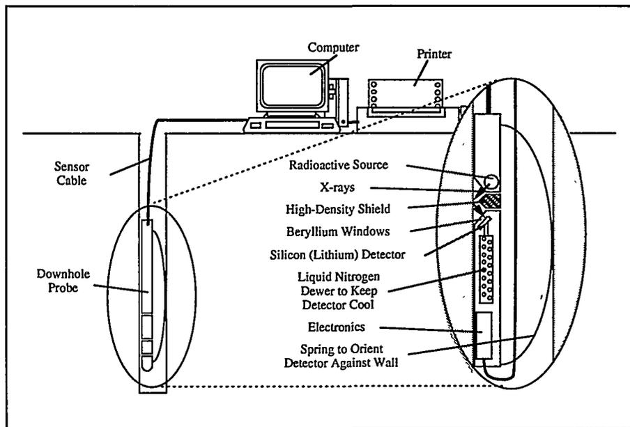
Prototype XRF System
