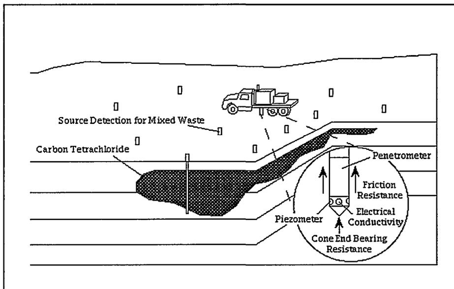
Source Detection Screening Using Cone Penetrometer
