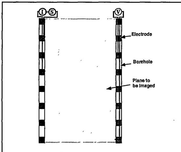
Figure 1. Schematic diagram showing the data collection approach for ERT measurements, where: I = source current, S = signal source, and V = voltage.
