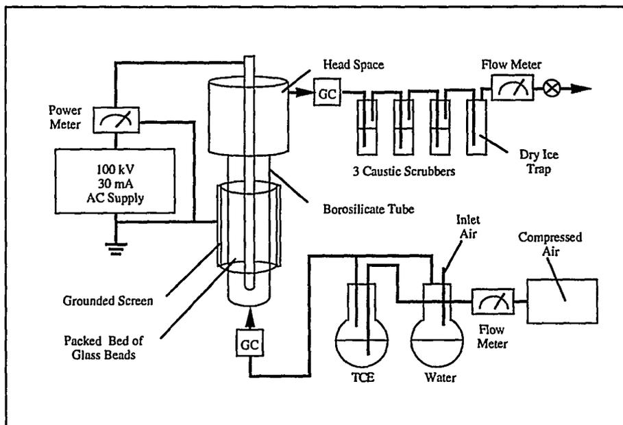
The technology is packaged in a self-contained mobile office that includes gas-handling equipment and on-line analytical capabilities. Site power is not absolutely required. Installation consists of connecting inlet and outlet hoses to the HEC process trailer. Training in the use of the equipment can usually be accomplished well within one hour. Failure control is provided by a combination of automated and manually activated means, addressing electri-
