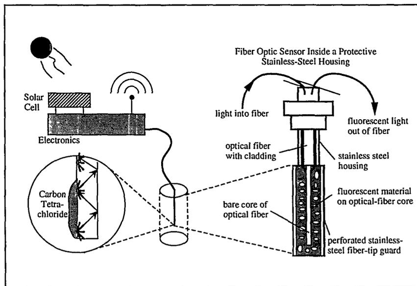
Figure 2. Reversible Fiber-Optic  $\text{CCl}_4$  Sensor
