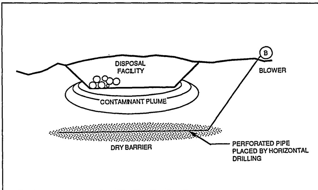
Figure 1. Schematic of a Dry Barrier for a Contaminant Plume
