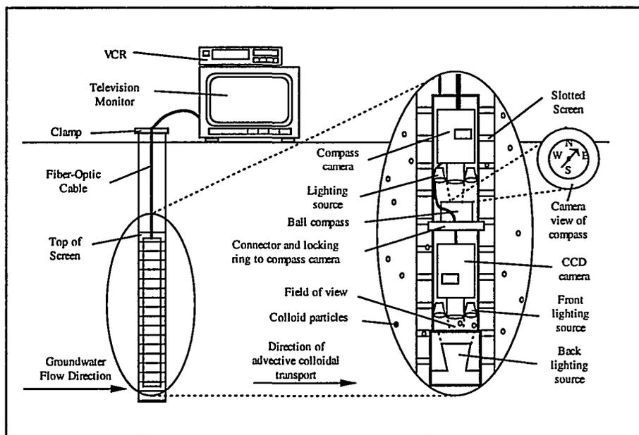
Cross-Section of a Boreoscope in a Well
