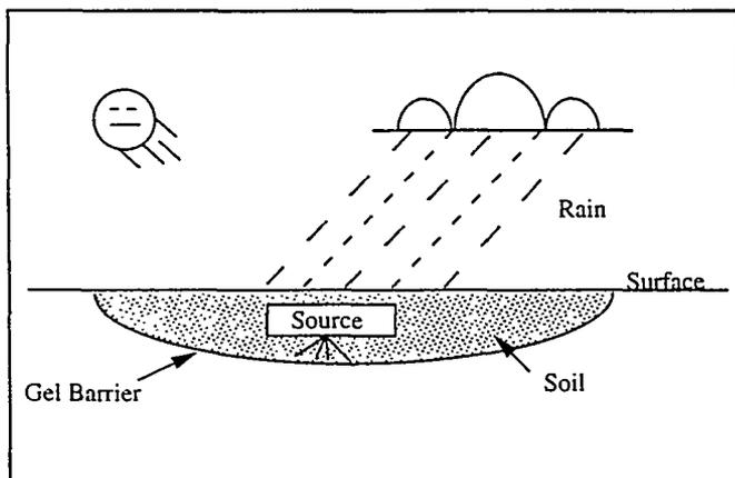
Figure 1. Gel Barrier for In Situ Use.
