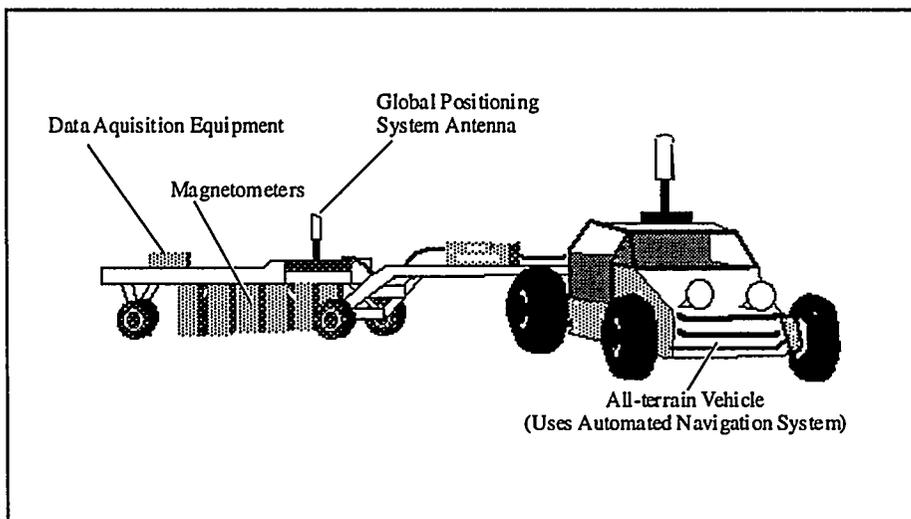
Magnetometer Towed Array
