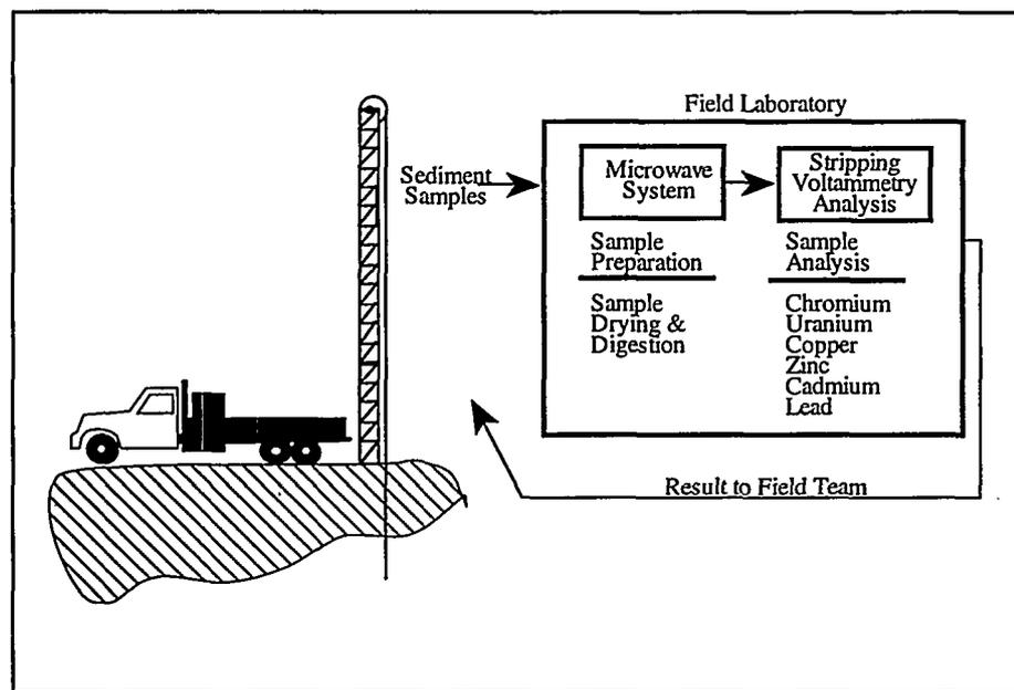
Adsorptive Stripping Voltammetry
