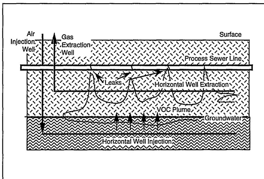
Schematic Diagram of Horizontal Well In Situ Air Stripping
