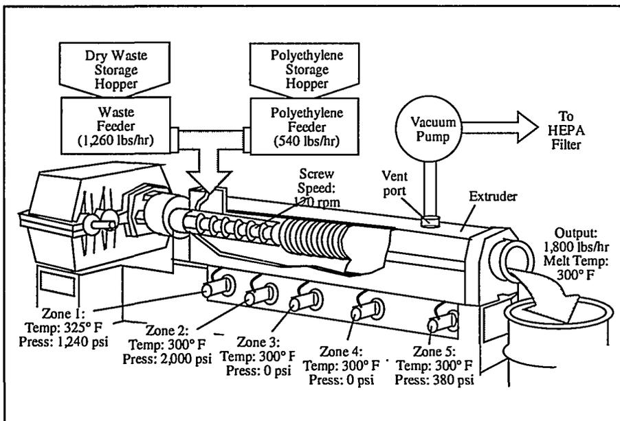
Polyethylene Encapsulation System
