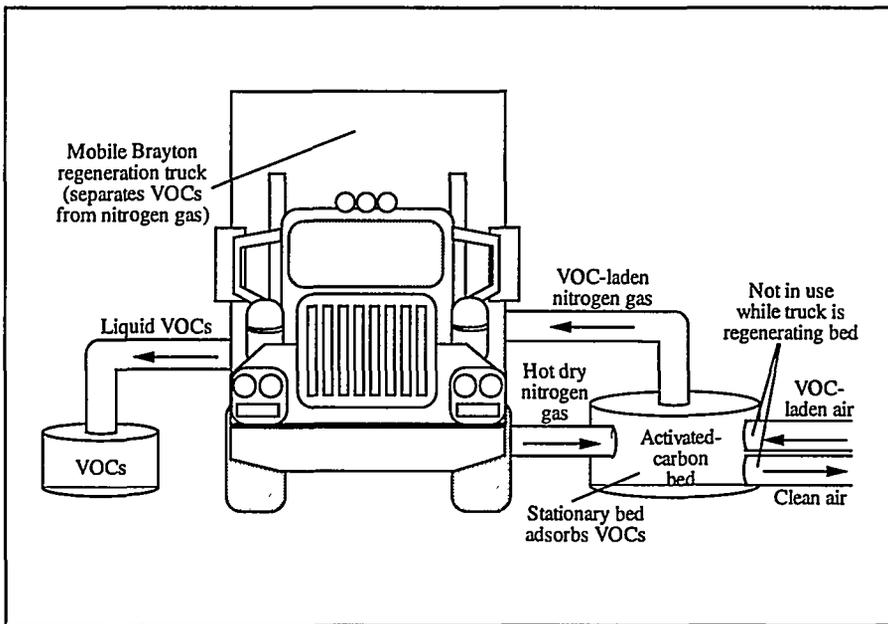
Decoupled Brayton-Cycle Solvent-Recovery Heat Pump for Small Emitters
