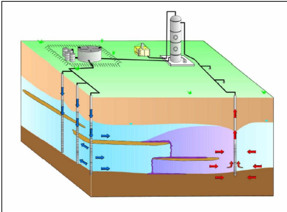
**Figure 2-1.** Conceptual Design of a Surfactant/Cosolvent Flushing System
