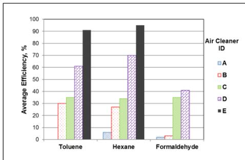
Figure 3. Initial efficiency test averages for the indoor gases (Owen et al., 2014a, b)
