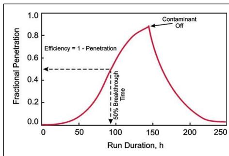
**Figure 2.** Typical sorbent breakthrough curve for carbon or other solid sorbents
