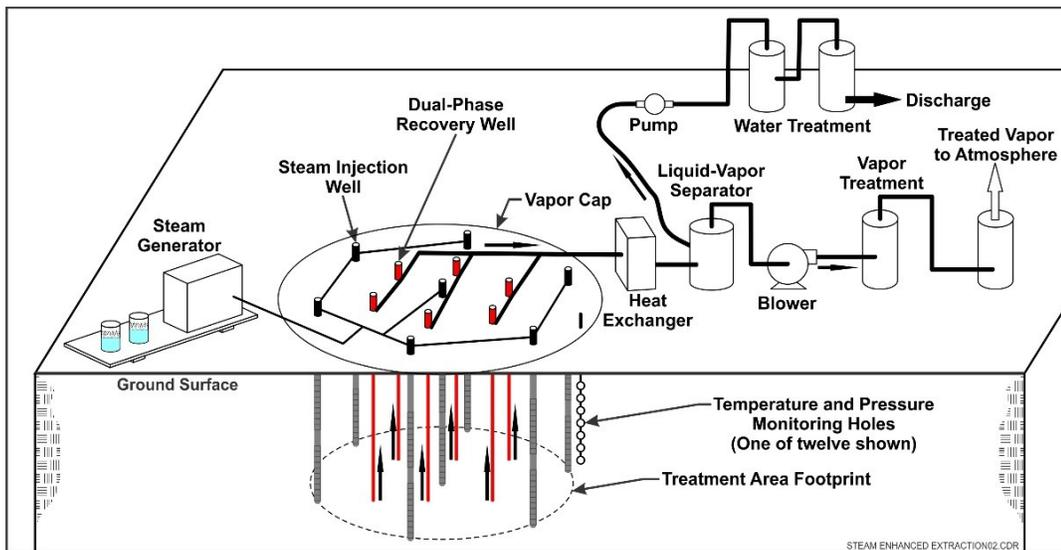
In Situ Steam Flooding Heating System
