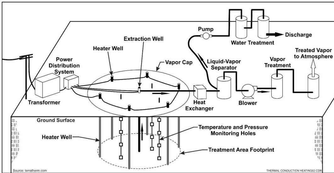
Thermal Conduction Heating System Schematic
