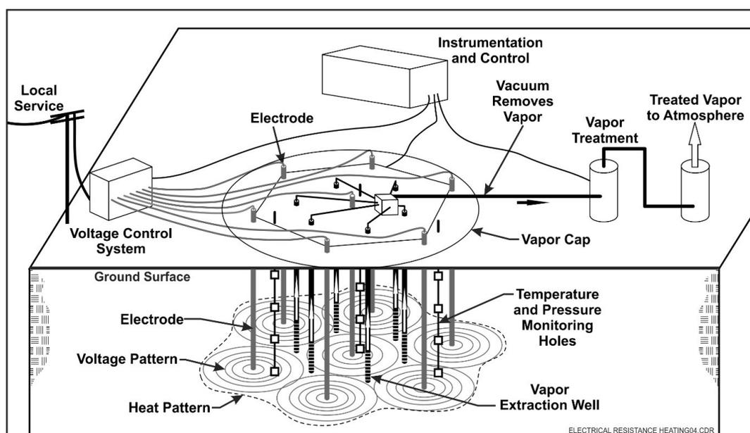
Electrical Resistance Heating System Schematic
