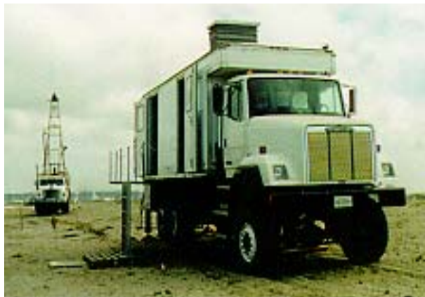
Figure 1. SCAPS Penetrometer Truck.
