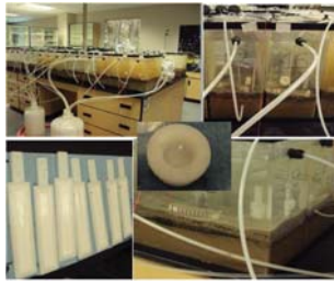
The bioavailable pool of metals in the water and sediment (capped and untreated) was measured by two types of diffusive gradients in thin films (DGT) probes
