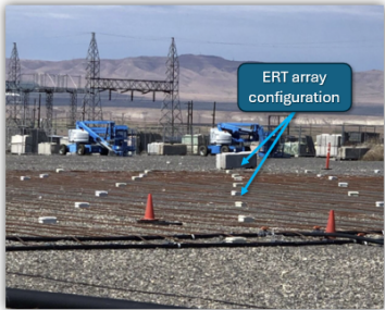
Electrode configuration for resistivity imaging used to monitor in situ soil flushing at the Hanford 100-K East Area (Johnson et al., 2024).
