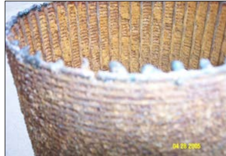
Well Screen with Metal Precipitates
