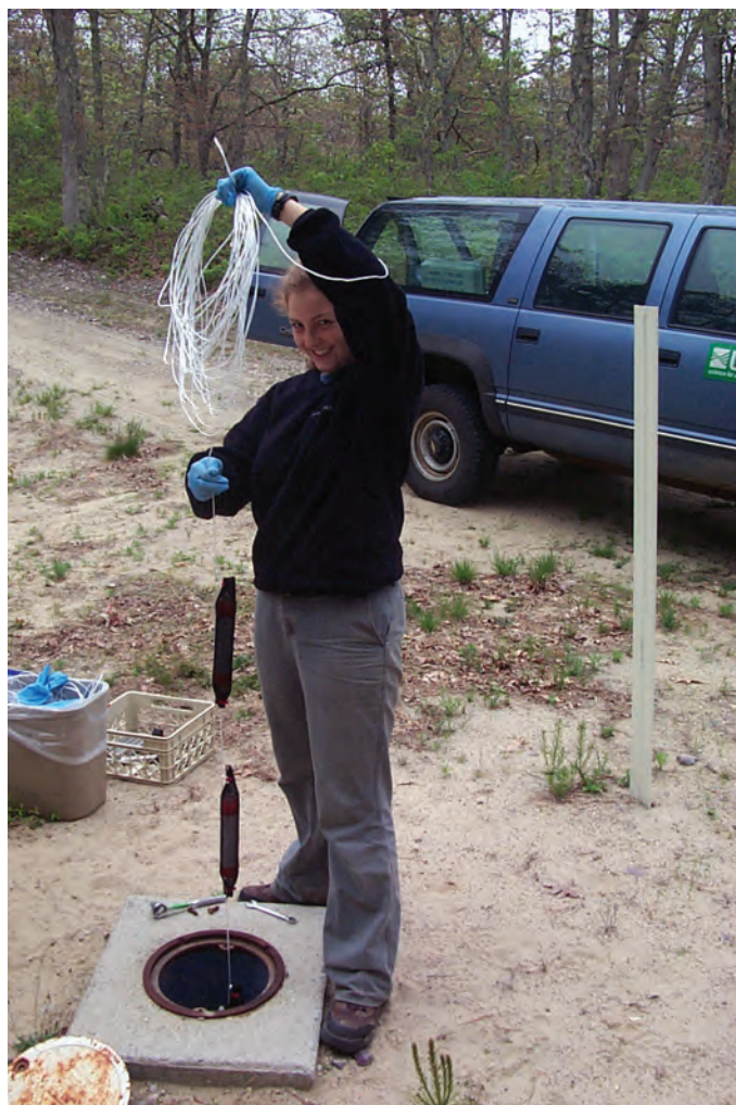
Figure 3. Vertical arrangement of diffusion samplers as they are retrieved from a well. Note flexible polyethylene mesh enclosing each diffusion sampler.
